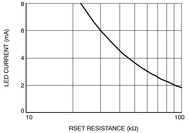
Figure 5. LED Current vs. RSET
