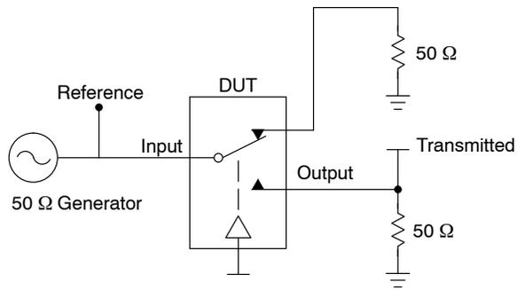
Channel switch control/s test socket is normalized. Off isolation is measured across an off channel. On loss is the bandwidth of an On switch.  $V_{ISO}$ , Bandwidth and  $V_{ONL}$  are independent of the input signal direction.
