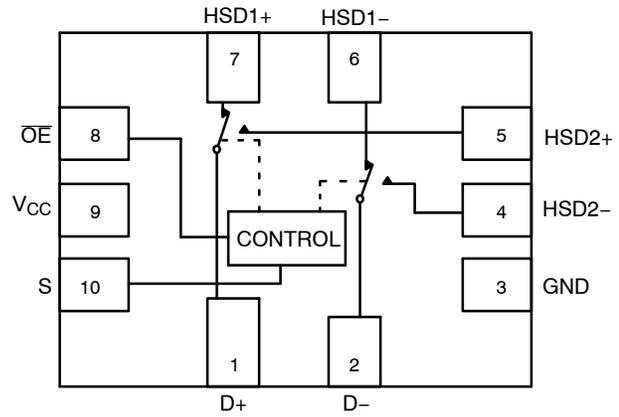
**Figure 2. Pin Connections and Logic Diagram**
