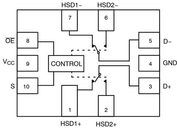
**Figure 1. Pin Connections and Logic Diagram**
