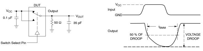
Figure 4. t<sub>BBM</sub> (Time Break-Before-Make)
