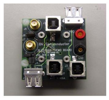
Figure 10. Photograph of the NLAS7222B USB Demo Board
