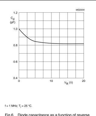
Fig.6 Diode capacitance as a function of reverse voltage; typical values.
