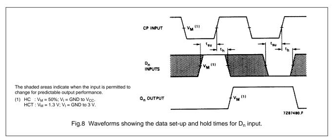
Octal D-type flip-flop; positive edge-trigger; 3-state
