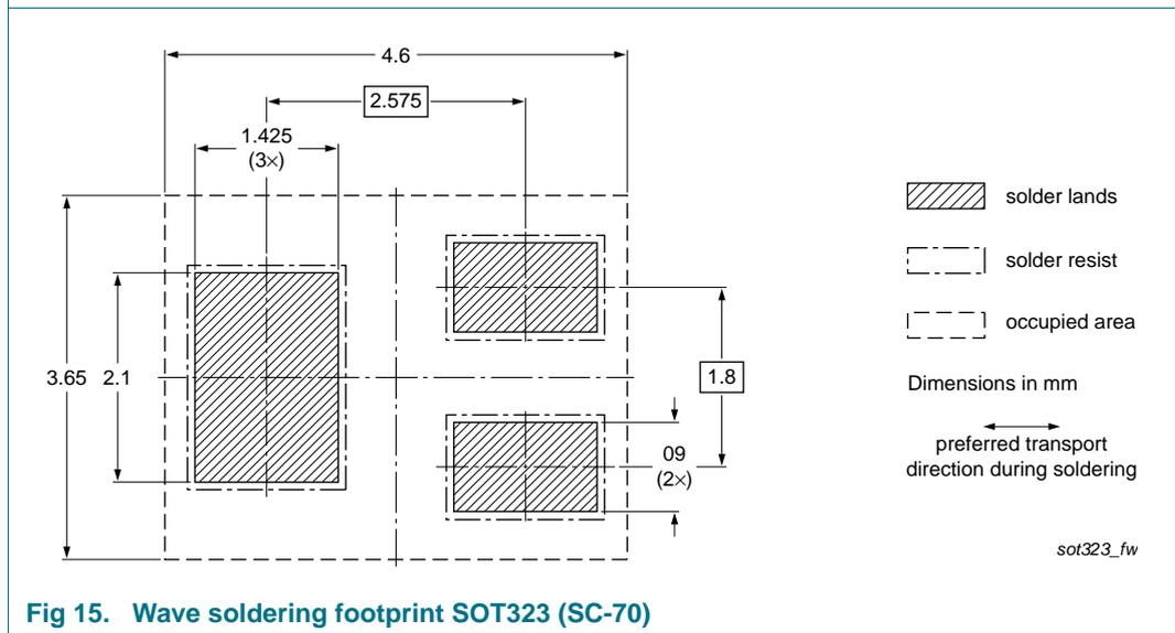
Fig 15. Wave soldering footprint SOT323 (SC-70)
