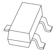
PBSS5120T 20 V, 1 A PNP low V<sub>CEsat</sub> (BISS) transistor
