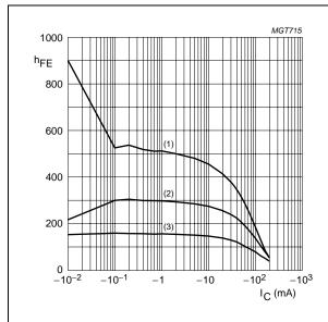
**BC857BW**;  $V_{CE} = -5 \text{ V}.$
