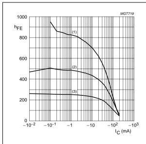
**BC857CW**;  $V_{CE} = -5 \text{ V}.$
