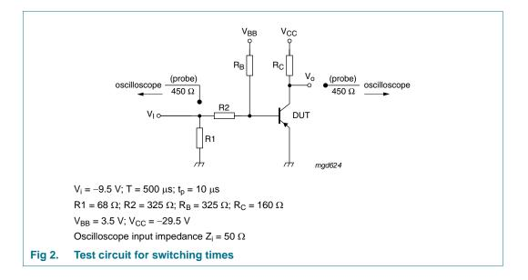
40 V, 600 mA PNP switching transistor
