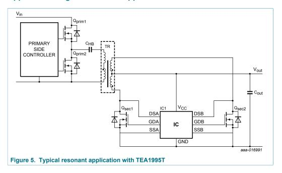
GreenChip dual synchronous rectifier controller
