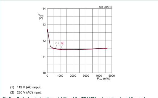
Fig 5. Typical output voltage stability of the TEA1721 universal mains white goods flyback controllers a function of load
