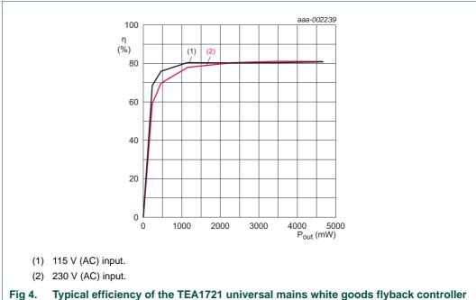
Fig 4. Typical efficiency of the TEA1721 universal mains white goods flyback controlle as a function of load
