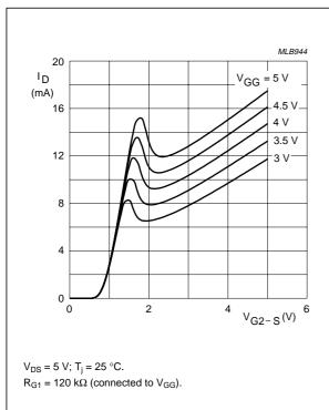
Fig.12 Drain current as a function of gate 2 voltage; typical values; see Fig.18.
