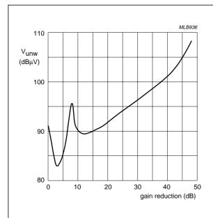
$V_{DS} = 5 \text{ V; } V_{GG} = 5 \text{ V; } f_w = 50 \text{ MHz.}$   $f_{unw} = 60 \text{ MHz; } T_{amb} = 25 \text{ °C; } R_{G1} = 120 \text{ k}\Omega.$
