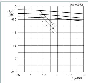
Diode inserted in series with a 50  $\Omega$  strip line circuit and biased via the analyzer T-network. T<sub>i</sub> = 25 °C; f = 1 MHz
