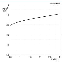
Diode zero-biased and inserted in series with a 50  $\Omega$  strip line circuit and biased via the analyzer T-network. T<sub>i</sub> = 25 °C; f = 1 MHz
