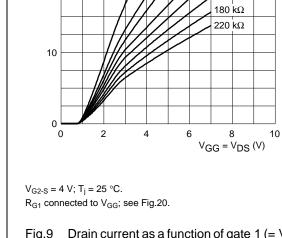
Fig.9 Drain current as a function of gate 1 (=  $V_{GG}$ ) and drain supply voltage; typical values.
