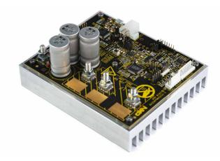
Figure 1: S12ZVM 3-phase motor control evaluation board
