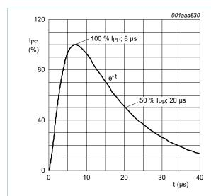
Fig. 2. 8/20 μs pulse waveform according to IEC 61000-4-5 and IEC 61643-321
