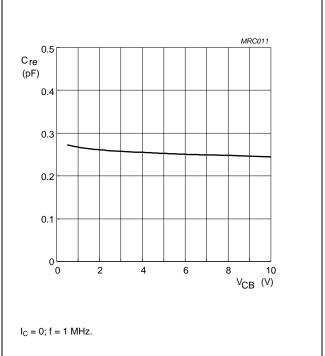
Fig.4 Feedback capacitance as a function of collector-base voltage.
