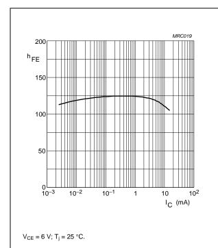
Fig.3 DC current gain as a function of collector current.
