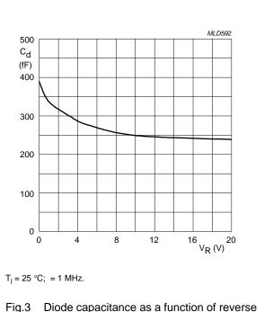
Fig.3 Diode capacitance as a function of reverse voltage; typical values.
