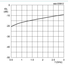
Diode zero-biased and inserted in series with a 50  $\Omega$  strip line circuit and biased via the analyzer T-network; T<sub>amb</sub> = 25 °C
