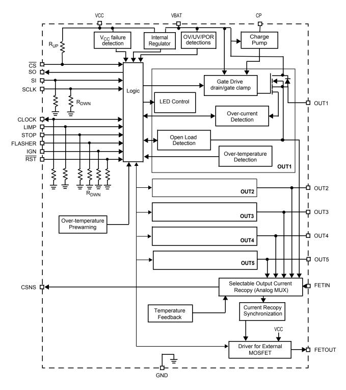
Figure 2. 35XS3500 Simplified Internal Block Diagram
