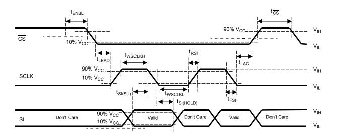
Figure 4. Input Timing Switching Characteristics
