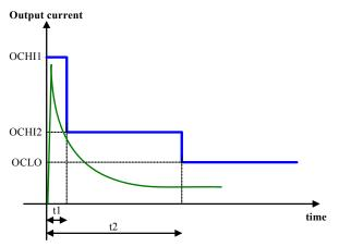
Figure 12. Double Over-current Window in Normal Mode
