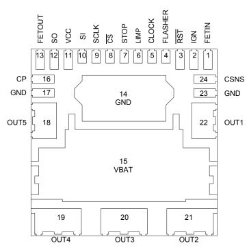
Figure 3. 35XS3500 Pin Connections (Transparent Package Top View)
