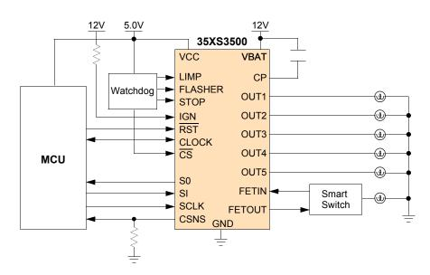
Figure 1. 35XS3500 Simplified Application Diagram
