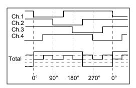
The synchronization of the switching phases between different corner light IC is provided by a SPI command in combination with the  $\overline{\text{CS}}$  input. The bit in the SPI is called PWM sync (initialization register).
