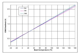
Figure 17. Analog Temperature Precision with Calibration Strategy
