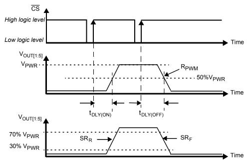
Figure 6. Output Slew Rate and Time Delays
