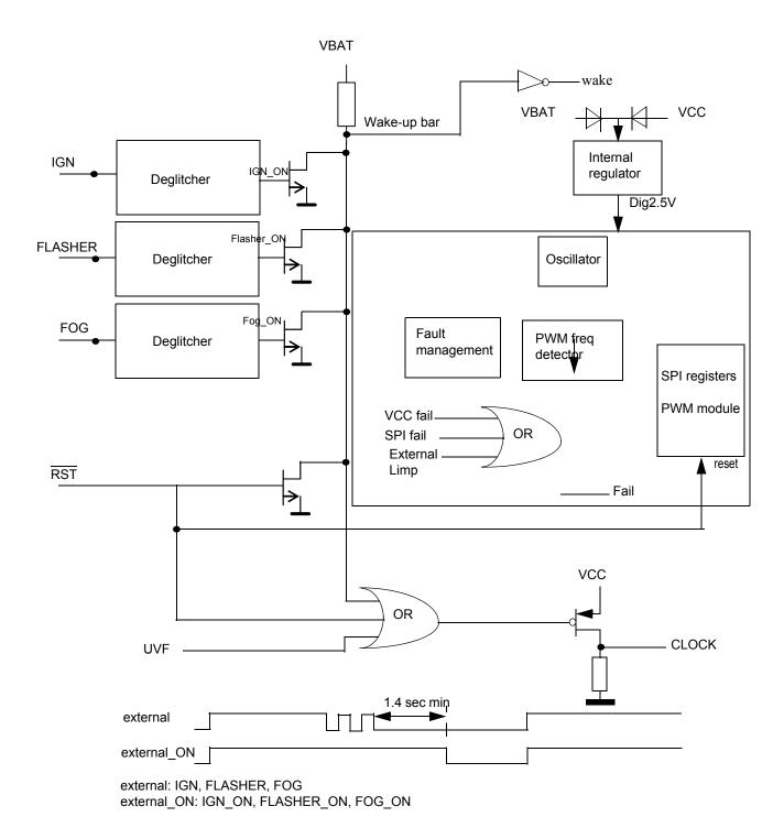
Figure 11. Wake-up Block Diagram
