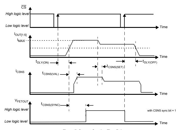
Figure 7. Current Sensing Time Delays
