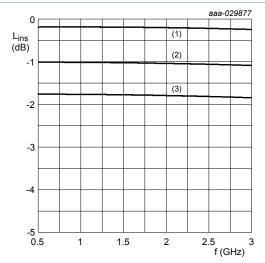
Diode inserted in series with a 50  $\Omega$  strip line circuit and biased via the analyzer T-network. T<sub>amb</sub> = 25  $^{\circ}C.$
