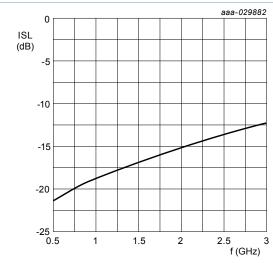
Diode zero biased and inserted in series with a 50  $\Omega$  strip line circuit.  $T_{amb}$  = 25  $^{\circ}C.$
