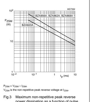
power dissipation as a function of pulse duration (square pulse).
