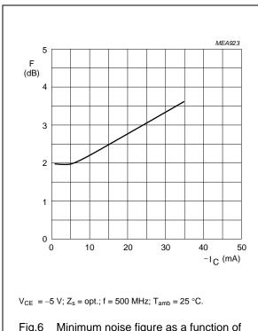
Fig.6 Minimum noise figure as a function of collector current.
