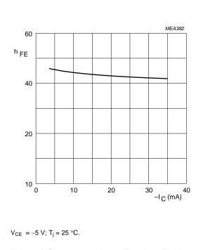
Fig.3 DC current gain as a function of collector current.
