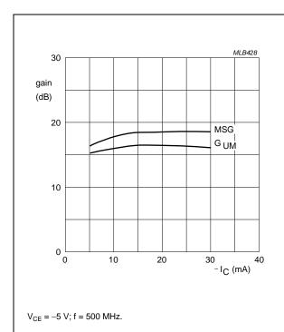
Fig.6 Gain as a function of collector current, typical values.
