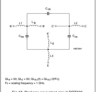
Fig.18 Package equivalent circuit SOT323.
