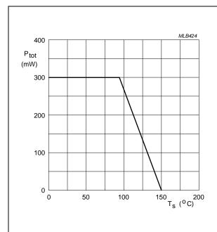
Fig.2 Power derating as a function of the soldering point temperature.
