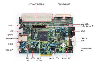
Figure 1: Top elevation of MPC5777C Development Board
