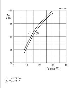
Fig.9 Intermodulation distortion as a function of peak synchronized output power.
