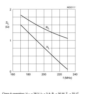
Class-A operation;  $V_{DS}$  = 28 V;  $I_{D}$  = 3 A;  $P_{L}$  = 30 W;  $T_{h}$  = 70 °C.
