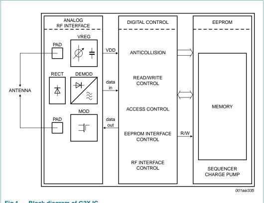
Fig 1. Block diagram of G2X IC
