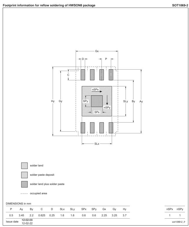
Fig 22. PCB footprint for SOT1069-2 (HWSON8); reflow soldering
