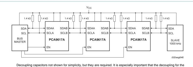
Decoupling capacitors not shown for simplicity, but they are required. It is especially important that the decoupling for the PCA9617A  $V_{CC(B)}$  be close to the  $V_{CC(B)}$  pin.
