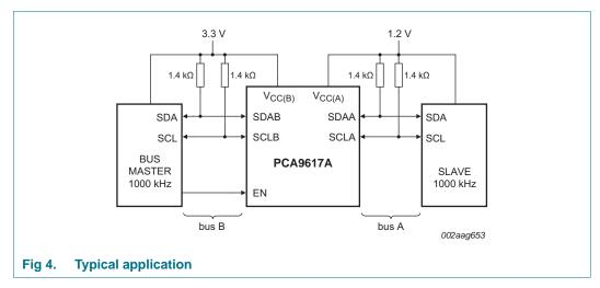
The PCA9617A is 5 V tolerant, so it does not require any additional circuitry to translate between 0.8 V to 5.5 V bus voltages and 2.2 V to 5.5 V bus voltages.
