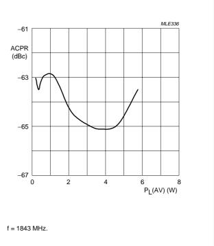
Fig.3 GSM EDGE ACPR at 400 kHz as a function of load power; typical values.
