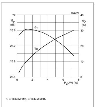
Fig.7 Two tone gain power and efficiency as functions of load power; typical values.
