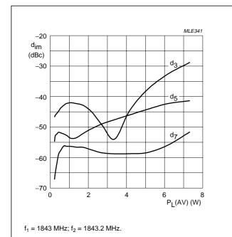
Fig.8 Two tone intermodulation distortion as a function of average load power; typical values.
