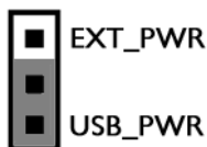
Figure 7-1: Power Source Selection Header (J3)
