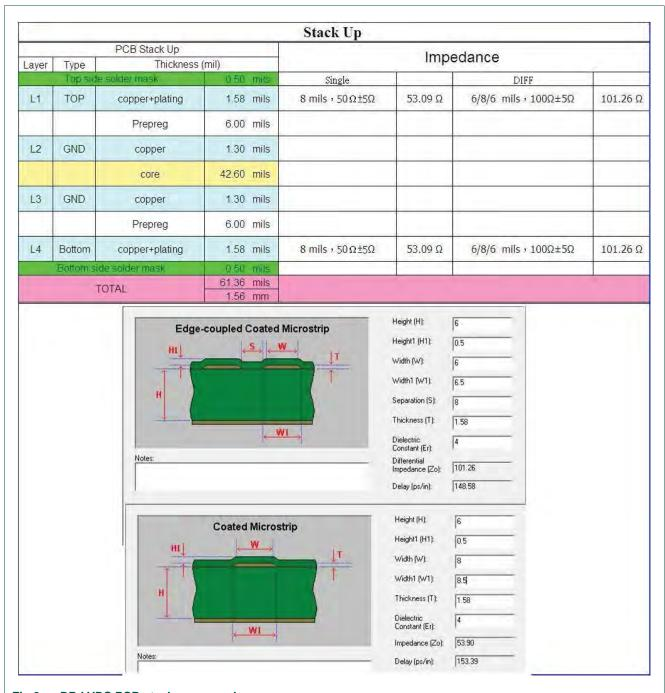
Fig 2. DP-LVDS PCB stack up example
