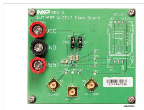
Fig 1. NVT4555UK SIM card voltage level translators evaluation board (OM13480)
