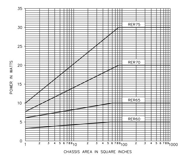
NOTE: The chassis derating curves are based on the full power ratings at an ambient temperature of 25 °C. These curves are independent of the temperature derating curves.
