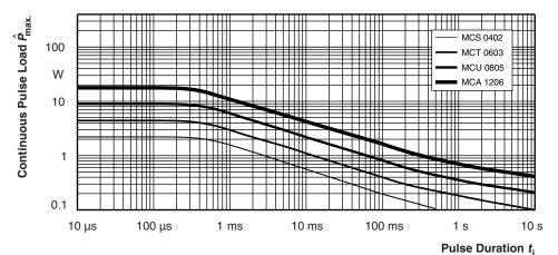
Maximum pulse load, continuous pulses; applicable if  $\bar{P} \leq P\left(\vartheta_{\rm amb}\right)$  and  $\hat{U} \leq \hat{U}_{\rm max}$ ; for permissible resistance change equivalent to 8000 h operation in standard operation mode
