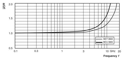
Relative impedance for 49.9  $\Omega$  chip resistor
