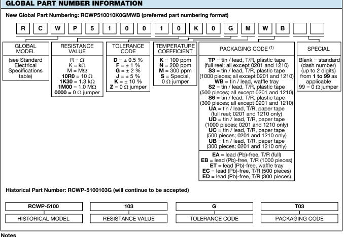
For additional information on packaging, refer to the Surface Mount Resistor Packaging document (<u>www.vishay.com/doc?31543</u>) Tape and reel packaging with plastic tape standard for all case sizes except 0201 and 1210. For the 0201 and 1210 case sizes, the product is only offered in tape and reel packaging with paper tape (1)
