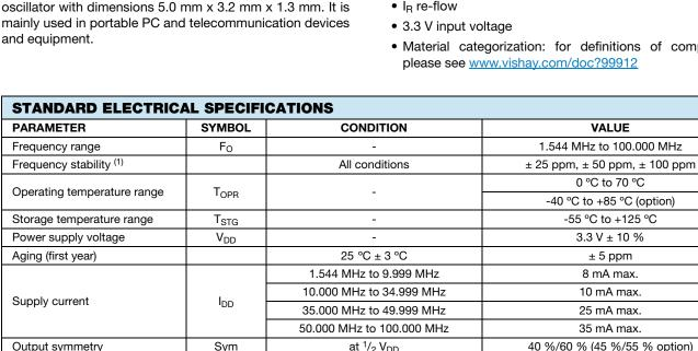
35 mA max. 40 %/60 % (45 %/55 % option) Output symmetry Sym at  $1/_2 V_{DD}$ Rise time tr 10 %  $V_{DD}$  to 90 %  $V_{DD}$ 7 ns max. Fall time 90 % V<sub>DD</sub> to 10 % V<sub>DD</sub> 7 ns max. t<sub>f</sub> VOH 90 % V<sub>DD</sub> min. Output voltage VOL \_ 10 % V<sub>DD</sub> max. Output load HCMOS load 30 pF max. (15 pF typ.) \_ Start-up time 10 ms max. ts \_ Pin 1 = H or open (output active at pin 3) Pin 1, tri-state function \_
