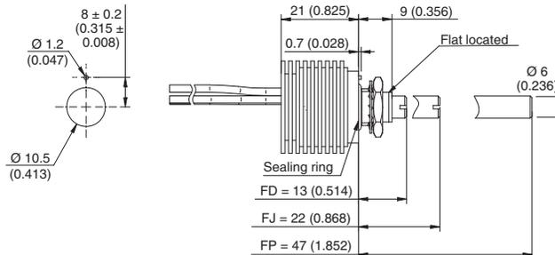
Available only with bushing M10 x 0.75 and shafts Ø 6 mm
