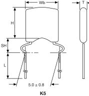
K2 Component outline for lead spacing 2.5 mm  $\pm$  0.8 mm lead spacing 5.0 mm  $\pm$  0.8 mm (outside kink)
