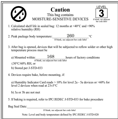
EIA JEDEC standard J-STD-020 level 3 label is included on all dry bags
