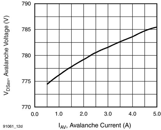
Fig. 13a - Typical Drain-to-Source Voltage vs. Avalanche Current
