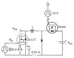
Fig. 12a - Unclamped Inductive Test Circuit
