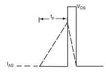
Fig. 12b - Unclamped Inductive Waveforms
