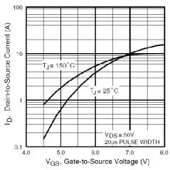
Fig. 3 - Typical Transfer Characteristics
