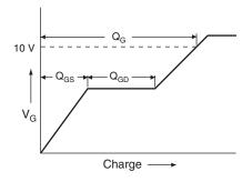
Fig. 12d - Basic Gate Charge Waveform
