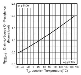
Fig. 4 - Normalized On-Resistance vs. Temperature
