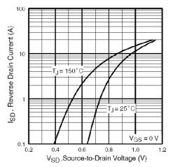
Fig. 7 - Typical Source-Drain Diode Forward Voltage
