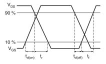
Fig. 10b - Switching Time Waveforms
