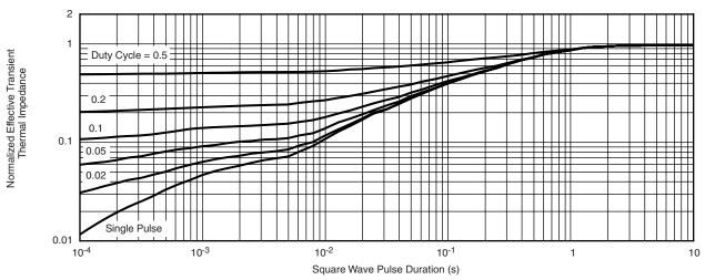
Normalized Thermal Transient Impedance, Junction-to-Foot
