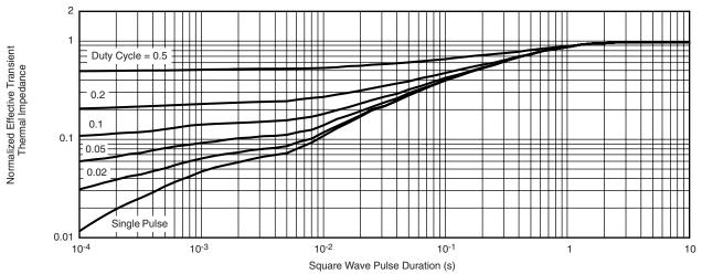
Normalized Thermal Transient Impedance, Junction-to-Foot
