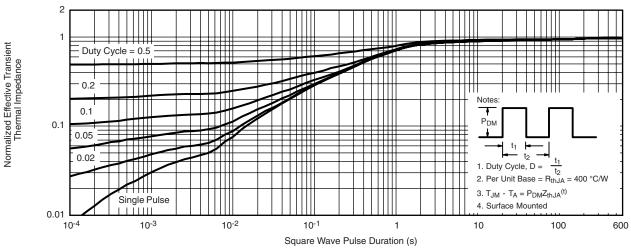
Normalized Thermal Transient Impedance, Junction-to-Ambient
