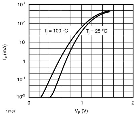
Fig. 1 - Forward Characteristics
