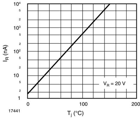
Fig. 5 - Leakage Current vs. Junction Temperature
