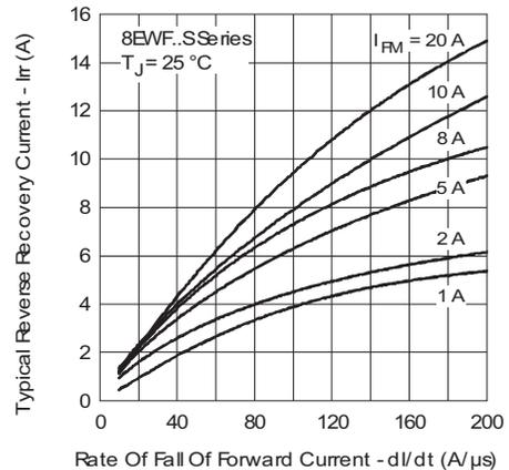
Fig. 12 - Recovery Current Characteristics,  $T_J = 25\text{ }^\circ\text{C}$
