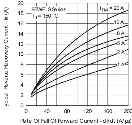
Fig. 13 - Recovery Current Characteristics,  $T_J = 150\text{ }^\circ\text{C}$
