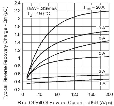
Fig. 11 - Recovery Charge Characteristics,  $T_J = 150\text{ }^\circ\text{C}$
