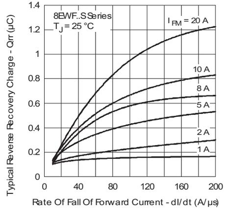
Fig. 10 - Recovery Charge Characteristics,  $T_J = 25\text{ }^\circ\text{C}$
