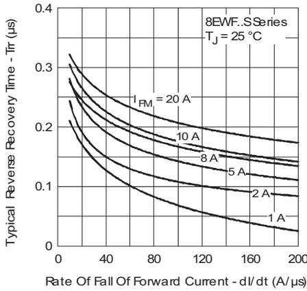
Fig. 8 - Recovery Time Characteristics,  $T_J = 25\text{ }^\circ\text{C}$
