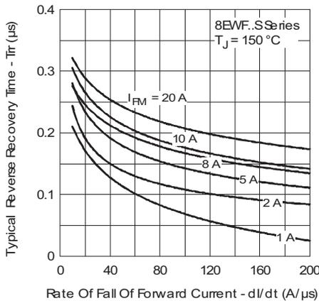
Fig. 9 - Recovery Time Characteristics,  $T_J = 150\text{ }^\circ\text{C}$
