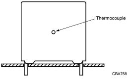
The temperature is measured in unloaded ( $T_{amb}$ ) and maximum loaded condition ( $T_C$ ). The temperature rise is given by  $\Delta T = T_C - T_{amb}$ .
