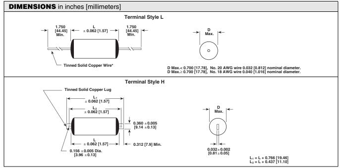
\* Leads to be within ± 0.062" [1.57 mm] of center line at egress but not less than 0.031" [0.79 mm] from edge (Terminal Style L only).
