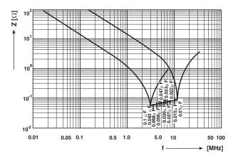
Impedance (Z) as a function of frequency (f) at  $T_a = 20$  °C (average). Measurement wiht lead length 6 mm.
