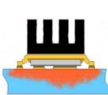
⑧ Mounted to a PCB with small clip heatsink (still air)
