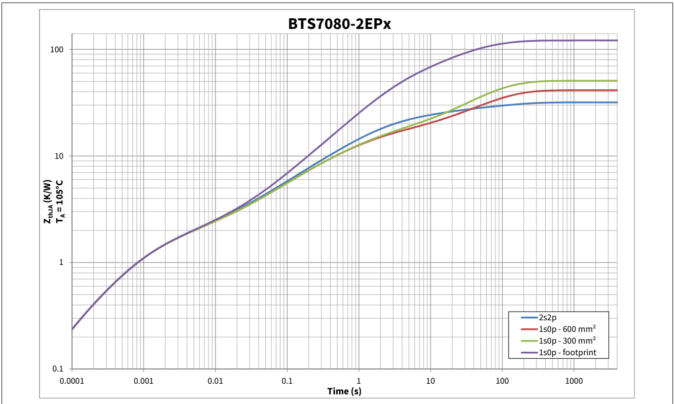
Figure 9 Typical Thermal Impedance. PCB setup according Chapter 4.4.1
