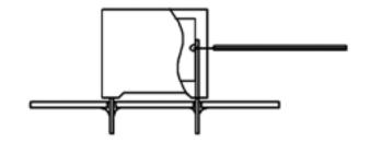
Temperature monitored inside the capacitor.
